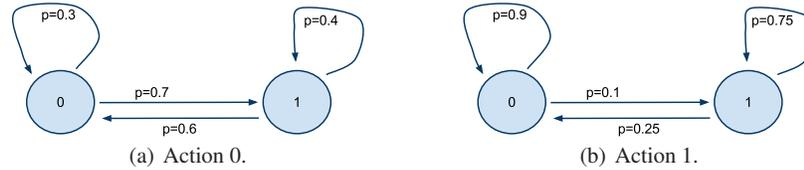
**Fig. 2** This figure shows the transition probabilities for a simple two state MDP for both actions 0 and 1. We assume a reward of -1 for transitions leading to state 0, and a reward of +1 for transitions leading to state 1.
