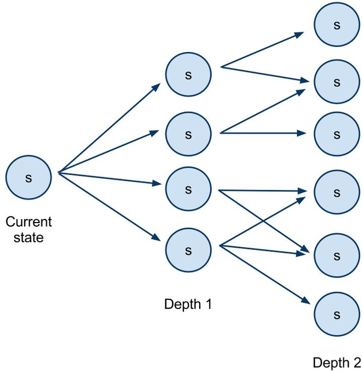
**Fig. 3** This figure shows a Monte Carlo Tree Search roll-out from the agent’s current state out to a depth of 2. The MCTS methods simulate a trajectory forward from the agent’s current state. At each state, they select some action, leading them to a next state one level deeper in the tree. After rolling out to a terminal state or a maximum depth, the value of the actions selected are updated towards the rewards received following it on that trajectory.
