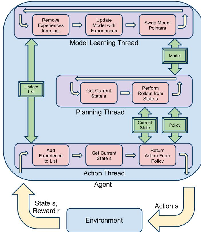
**Fig. 5** The parallel architecture for real-time model-based RL proposed by Hester et al (2011). There are three separate parallel threads for model learning, planning, and acting. Separating model learning and planning from the action selection enables it to occur at the desired rate regardless of the time taken for model learning or planning.
