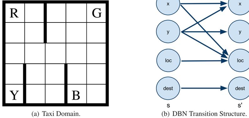
**Fig. 6** 6(a) shows the Taxi domain. 6(b) shows the DBN transition model for this domain. Here the  $x$  feature in state  $s'$  is only dependent on the  $x$  and  $y$  features in state  $s$  and the  $y$  feature is only dependent on the previous  $y$ . The passenger's *destination* is only dependent on its previous *destination*, and her current *location* is dependent on her location the step before as well as the taxi's  $x,y$  location the step before.
