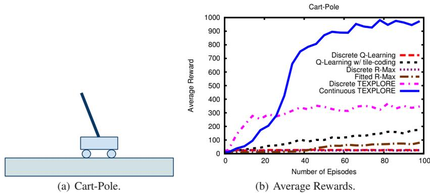
**Fig. 10** 10(a) shows the Cart-Pole Balancing task. 10(b) shows the average reward per episode for the algorithms on Cart-Pole Balancing averaged over 30 trials.
