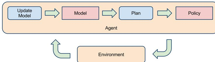
**Fig. 4** Typically, model-based agent's interleave model learning and planning sequentially, first completing an update to the model, and then planning on the updated model to compute a policy.
