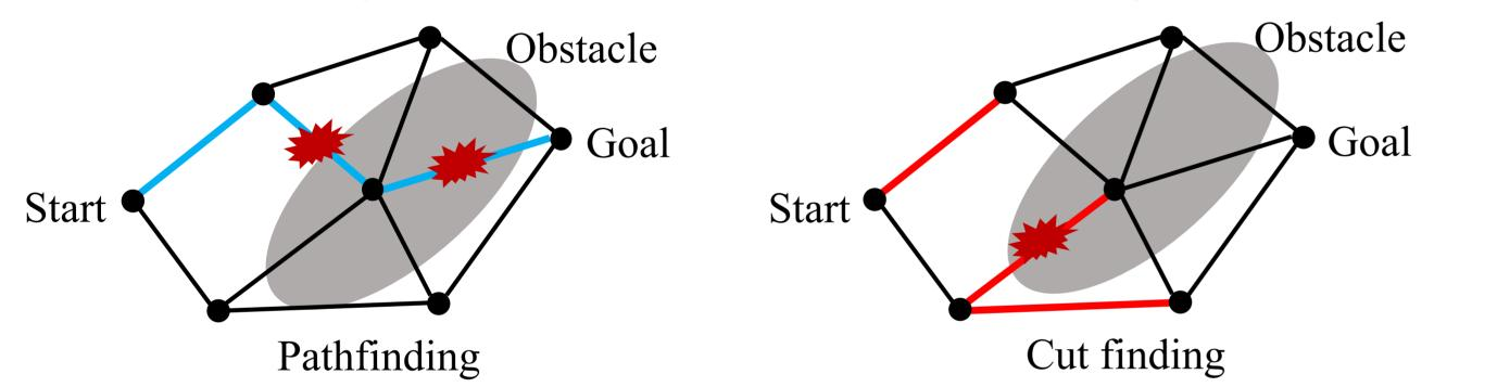
Cut finding is generally more expensive than pathfinding; we leverage the fact that cut finding separates the roadmap into two
