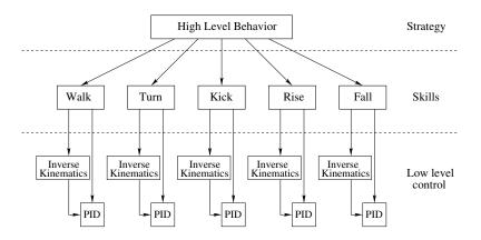
Figure 2. Schematic view of agent control architecture.
