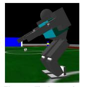
Figure 3. The humanoid is more stable when bent forward.
