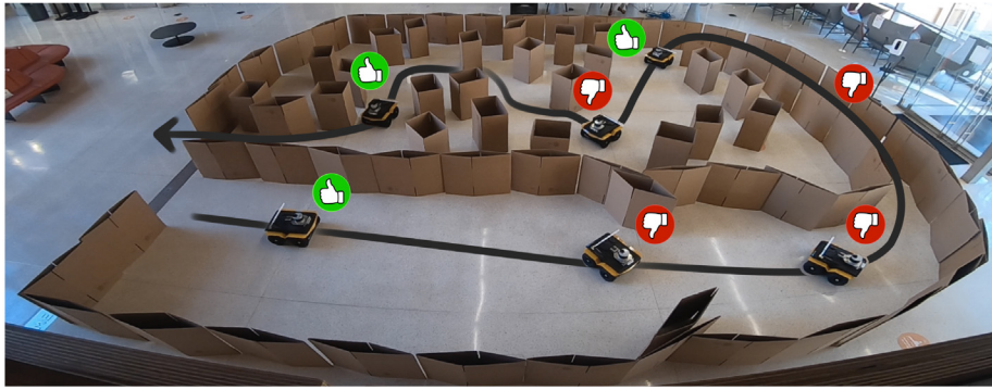
Fig. 7. For non-expert users who are unable or unwilling to take control of the robot, evaluative feedback, e.g. good job (green thumbs up) or bad job (red thumbs down), is a more accessible human interaction modality, but still valuable for improving navigation systems during deployment.
