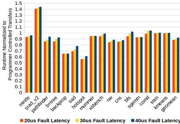
Figure 8: Sensitivity to increasing the end-to-end latency of constructing and servicing a transfer set.
