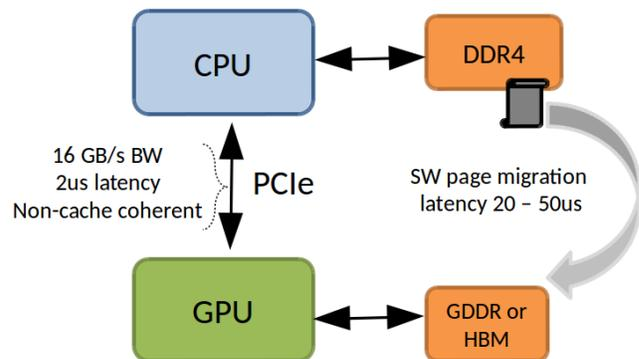
Figure 1: PCIe attached CPUs and GPUs implementing on-demand memory migration to the GPU.
