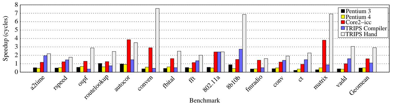
Figure 16: Speedup of TRIPS relative to the Core 2 on simple benchmarks.
