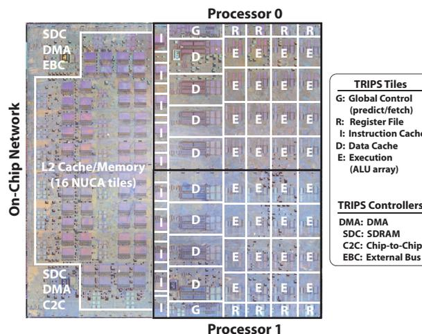
Figure 2: TRIPS die photo with tile overlays.
