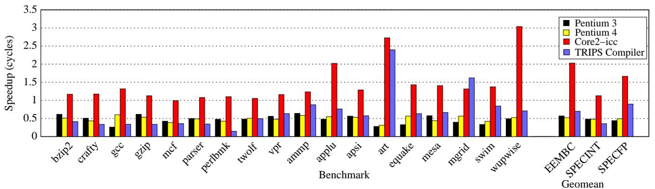
Figure 17: Speedup of TRIPS relative to the Core 2 on SPEC benchmarks.
