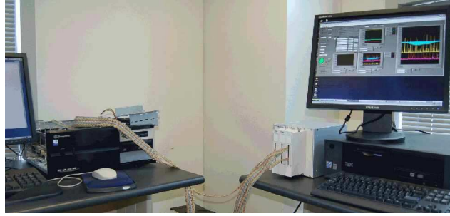
Figure 1: Equipment: Pentium M on left, data acquisition module and measurement PC with virtual oscilloscope on right
