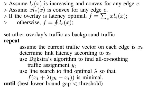
Fig. 2. The linear approximation algorithm to compute the best response of source routing or overlay routing, when the network is symmetric, assuming the other overlay's traffic is background.
