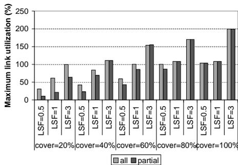
Fig. 13. Effects of partial coverage in *ISPT<sub>opto</sub>* with random node selection on maximum link utilization.
