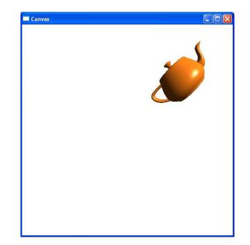
glMatrixMode (GL\_MODELVIEW); glMatrixMode (GL\_PROJECTION); glLoadIdentity(); glFrustum(-1, 1, -1, 1, 2, 7); glFrustum(-3, 1, -3, 1, 2, 7); glMatrixMode (GL\_MODELVIEW); glMatrixMode (GL\_MODELVIEW); glutSolidTeapot(1);
