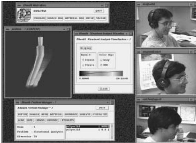
Figure 5: Stress Transfer Computation from Prosthesis to Femur in BHAUTIK
