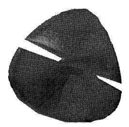
Figure 1: Missing points due to infinite parameter values
