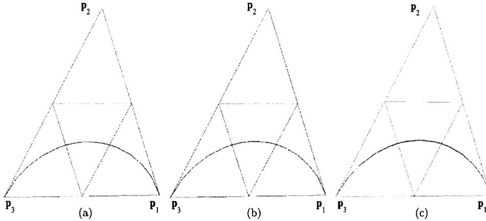
Fig. 4. In these figures  $\mathbf{p}_1 = (1, 0)T$ ,  $\mathbf{p}_2 = (3/5, 6/5)T$ , and  $\mathbf{p}_3 = (0, 0)T$  in Cartesian coordinates. (a): The exact energy-minimizing quadratic A-spline (4.16), with  $C^1$  continuity at the endpoints, obtained when  $b_{101} = 0.356$ . (b) The simplified energy-minimizing A-spline (4.19), obtained when  $b_{101} = 0.366$ . (c) Superposition of the curves in (a) and (b).
