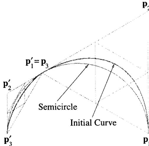
Fig. 5. Initial configuration. The point  $\mathbf{p}_3 = \mathbf{p}'_1$  is allowed to slide along the semicircle. The spline labeled “initial curve” is a typical minimal-energy spline if  $\mathbf{p}_3 = \mathbf{p}'_1$  is at the location indicated.
