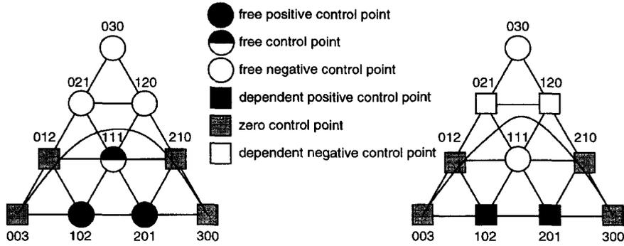
Fig. 2. Sign inequalities for the coefficients of (left)  $C^1$  and (right)  $C^3$  cubic A-splines. For  $i + j + k = 3$ , the symbol labeled by  $ijk$  indicates the sign restriction, if any, for the coefficient  $b_{ijk}$ .
