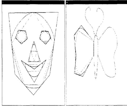
Fig. 1. Interactively designed contours with cubic A-splines.
