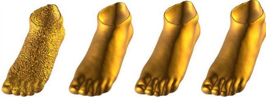
**Fig. 4.** *The left figure is the initial geometry mesh. The second figure is the faired mesh after 3 fairing iterations with uniform timestep  $t = 0.0011$ . The third and fourth figures are the faired meshes after 3 fairing iterations with adaptive timestep and alternatively adaptive diffusion tensor with uniform timestep  $\tau = 0.025$ , respectively.*
