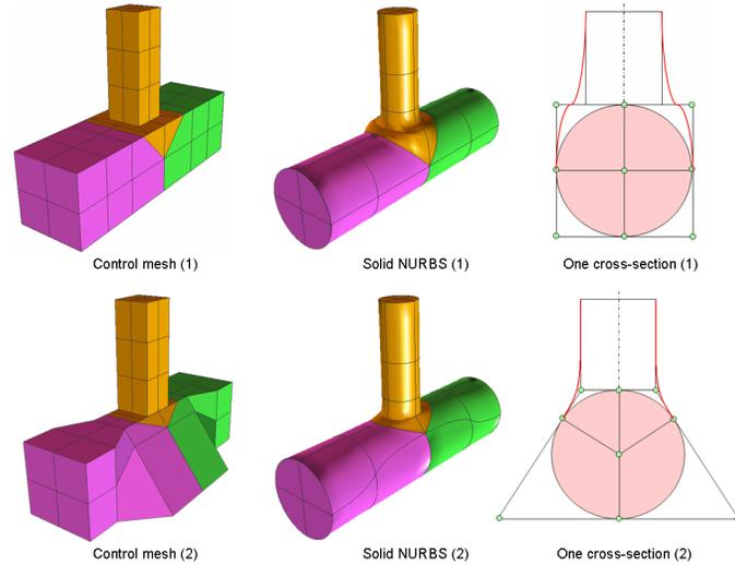
**Fig. 6.** Comparison of two meshes for the situation when the master branch and the slave branch have different diameters. Control nodes on cross-sections are distributed evenly in Mesh (1) (the top row), and unevenly in Mesh (2) (the bottom row). The red curves in the right two pictures are transition curves.
