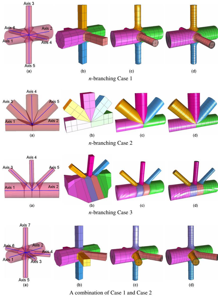
**Fig. 9.** The *n*-branching templates of Case 1-3 and a combination of Case 1-2. (a) - path; (b) - control mesh; (c) - solid NURBS; (d) - piecewise linear hex mesh. The Trifurcation geometry is decomposed into 6 patches (Case 1), 5 patches (Case 2) or 7 patches (Case 3, a combination of Case 1 and Case 2). Each patch is rendered with a different color.
