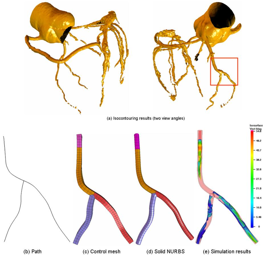
**Fig. 11.** Coronary artery. (a) - isocontouring results (two different view angles); (b) - path; (c) - control mesh; (d) - solid NURBS model (20,824 elements); (e) - rigid wall simulation results: isosurface of the drug concentration at 50% colored by the blood velocity magnitude (cm/s).
