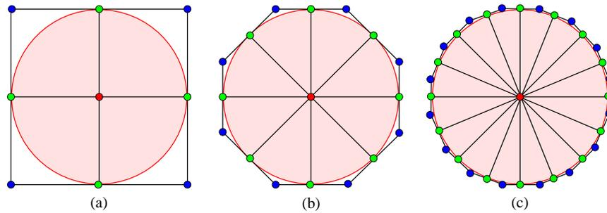
**Fig. 3.** Multi-resolution templates for cross-sections. (a) Level-1-template (9 control nodes); (b) Level-2-template (17 control nodes); (c) Level-3-template (25 control nodes). Red points are circle centers, green points are interpolatory control nodes on the circle, and blue points are non-interpolatory control nodes defined as the intersection point of two tangent lines at its two neighboring green points.
