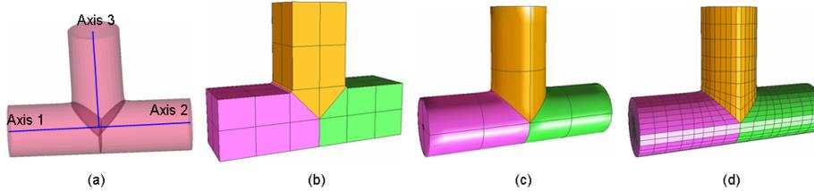
**Fig. 5.** The bifurcation decomposition template. (a) - path; (b) - control mesh; (c) - solid NURBS; (d) - a piecewise linear hex mesh. The bifurcation geometry is decomposed into 3 patches, and each patch is rendered with a different color.
