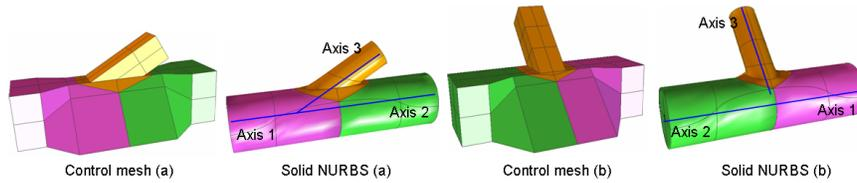
**Fig. 7.** Control mesh and solid NURBS (a) - the axes of the master and slave branches are not perpendicular to each other; Control mesh and solid NURBS (b) - the axes of the master and slave branches are not coplanar.
