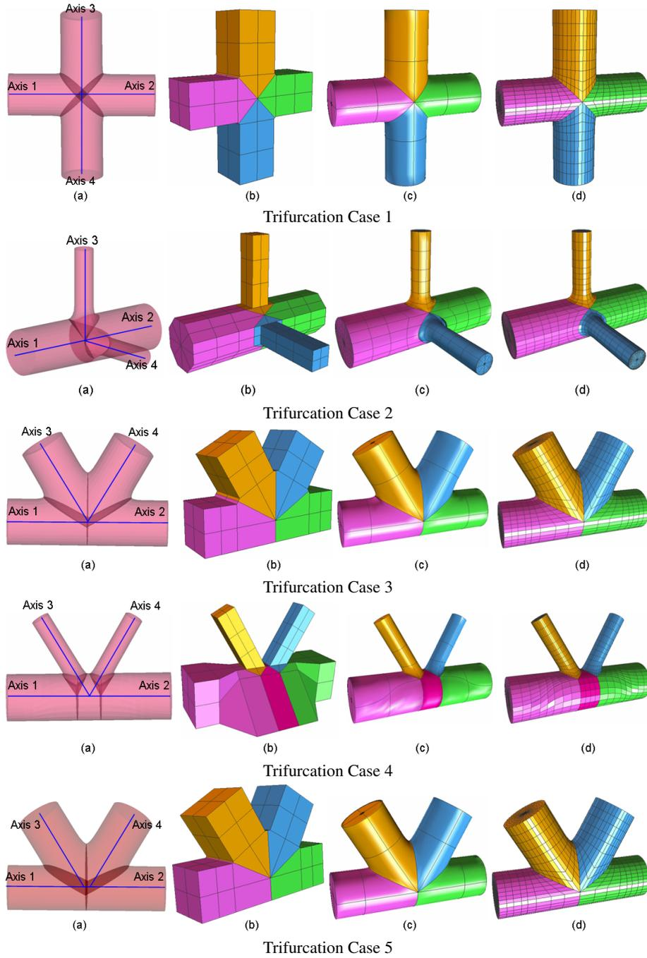
**Fig. 8.** The trifurcation decomposition templates of Case 1-4. (a) - path; (b) - hex control mesh; (c) - solid NURBS; (d) - piecewise linear hex mesh. The Trifurcation geometry is decomposed into 4 patches (Case 1, 2, 3, 5) or 5 patches (Case 4). Each patch is rendered with a different color.
