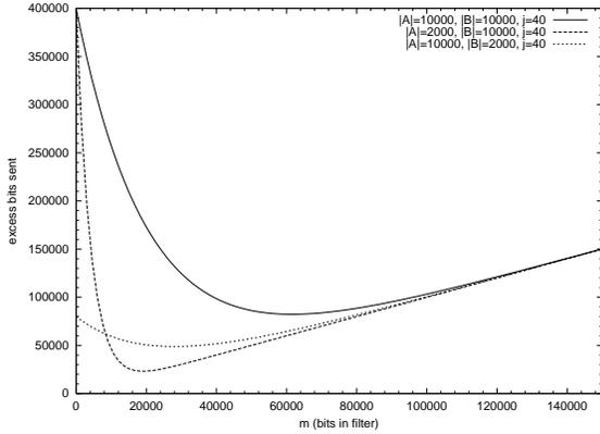
Figure 5: Expected excess bits sent as a function of  $m$
