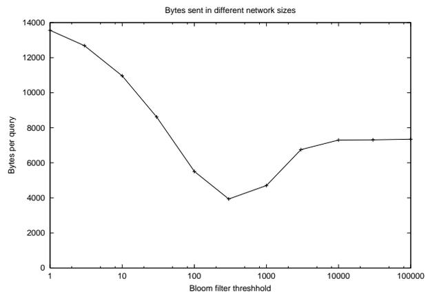
Figure 12: Increasing the Bloom filter threshold – i.e., using Bloom filters less often – significantly reduces the amount of data sent by eliminating the need to revisit nodes to eliminate false positives in certain cases.
