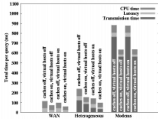
Figure 15: Isolating the effects of caching, virtual hosts, and different network characteristics for optimal Bloom threshold (300) and Bloom filter sizes (18/24 for caching on or off).
