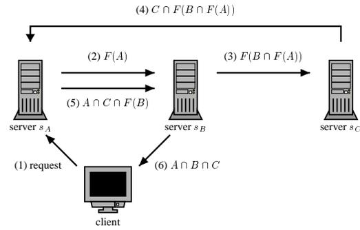
Figure 6: Using Bloom filters for more than two keywords
