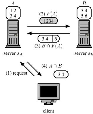
Figure 4: Bloom filters help reduce the bandwidth requirement of “AND” queries. The gray box represents the Bloom filter  $F(A)$  of the set  $A$ . Note the false positive in the set  $B \cap F(A)$  that server  $s_B$  sends back to server  $s_A$ .
