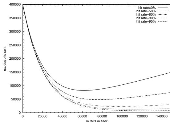
Figure 8: Improving cache hit rates reduces the amount of data sent and increases the size of the optimal Bloom filter.
