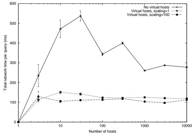
Figure 11: Virtual hosts cut the amount of time spent transmitting by up to 60%. Scaling the number of virtual hosts yields a small additional improvement.
