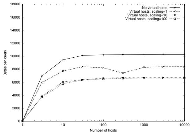
Figure 10: The number of bytes sent increases very little beyond networks of 100 hosts. Enabling virtual hosts reduces the number of bytes sent by about 18%. Scaling the number of virtual hosts reduces the number of bytes sent by an additional 18%.
