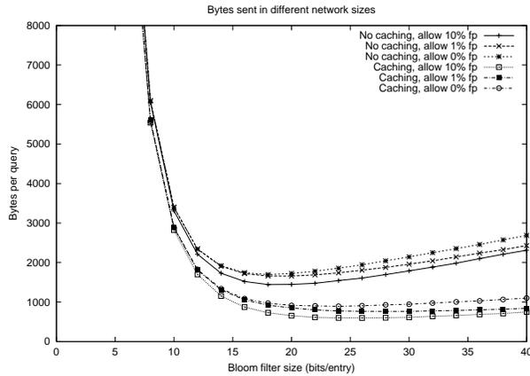
Figure 13: Bytes per query as a function of the Bloom filter size
