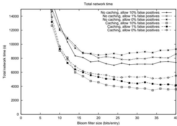
Figure 14: Network time (latency plus transmission time) per query as a function of the Bloom filter size
