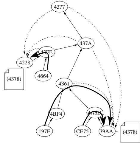
**Figure 3: Routing in Tapestry: Three different location requests.** For instance, to locate GUID 4378, query source 197E routes towards the root, checking for a pointer at each step. At node 4361, it encounters a pointer to server 39AA.
