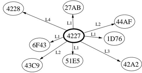
**Figure 1: Tapestry Routing Mesh.** Each node is linked to other nodes via *neighbor links*, shown as solid arrows with labels. Labels denote which digit is resolved during link traversal. Here, node 4227 has an L1 link to 27AB, resolving the first digit, an L2 link to 44AF, resolving the second digit, etc. Using the notation of Section 2.1, 42A2 is a (42, A) neighbor of 4227.
