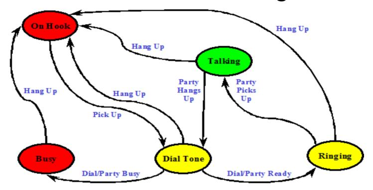
OnHook <*PickUP*> DialTone ... sequence (from previous slide) has 15 inputs, achieves *action coverage*: every action possible at each state "executed" at least once; *easiest test coverage criterion for FSM model*
