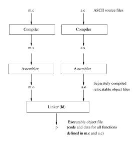
**Linking** is the process of combining various pieces of code and data into a single file that can be *loaded* (copied) into memory and executed.
