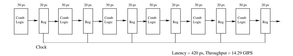
As you try to deepen the pipeline, the overhead of loading registers becomes more significant.
