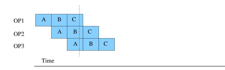
Up to 3 operations in process simultaneously.
