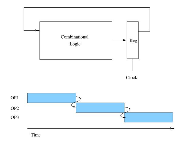
**Sequential System:** Each operation may depend on the previous one. (It doesn't matter for a sequential system. Why not?)
