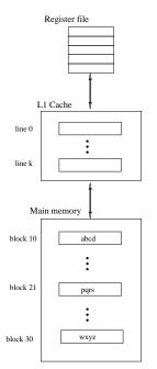
The tiny, very fast CPU register file has room for a small number of 8-byte words.
