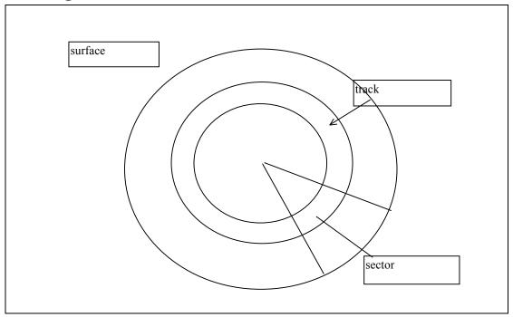
Disk **surface**: circular disk, coated with magnetic material **Tracks**: concentric rings around disk surface, bits laid out serially along each track
