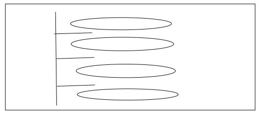
Disk is read/write via a comb - 2 read/write "heads" at end of each "arm"
