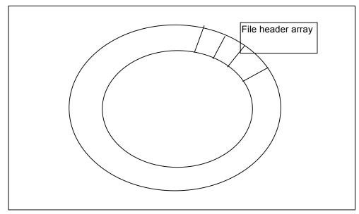
Unix refers to file by index into array – tells it where to find the file header
