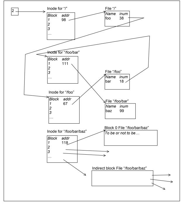
How many disk I/Os needed to access first byte of file
