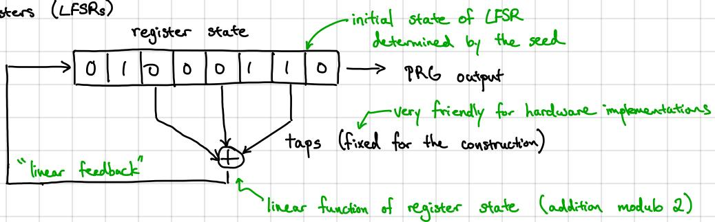
Each iteration: rightmost bit is output by LFSR
