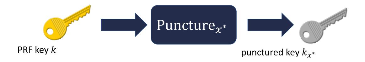
Punctured key  $k_{x^*}$  can be used to evaluate PRF on all points  $x \neq x^*$
