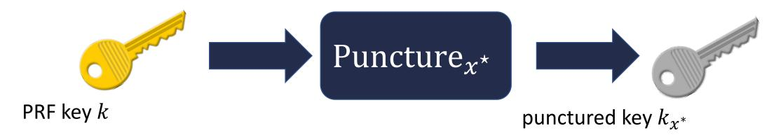
Punctured key  $k_{x^*}$  can be used to evaluate PRF on all points  $x \neq x^*$ (value at  $x^*$  is pseudorandom even given  $k_{x^*}$ )
