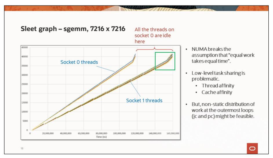
But, this asymmetry means that all the threads on socket 0 finish and then sit idle.
