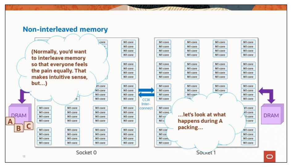
If memory is not interleaved, then the operand matrices (A, B, & C) would most likely all live on socket 0's DRAM, because that's where the primary thread that created them most likely lives. But, that leads to an unfair asymmetry: the cores on socket 1 are always experiencing longer latencies, while the cores on socket 0 are always experiencing shorter latencies.
