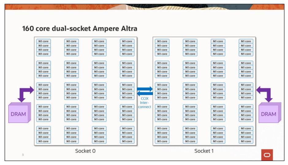
160 Neoverse N1 ARM cores on 2 sockets. 1 thread pinned to each core.
