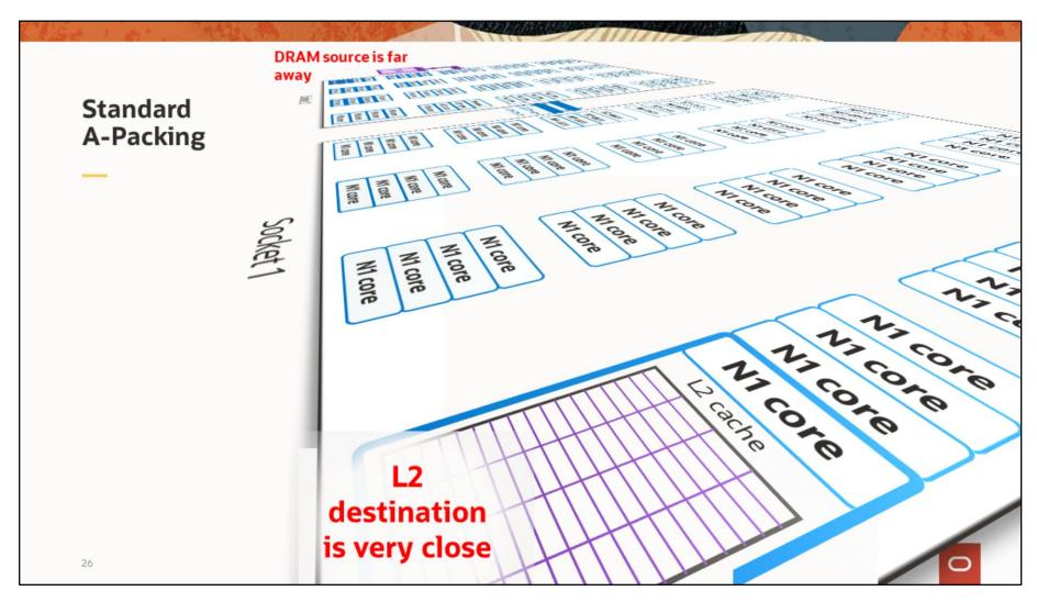
During A packing, the cores on socket 1 are reading data from the socket 0 DRAM which is *far away*, and writing to their own L2 cache which is *very close by*.
