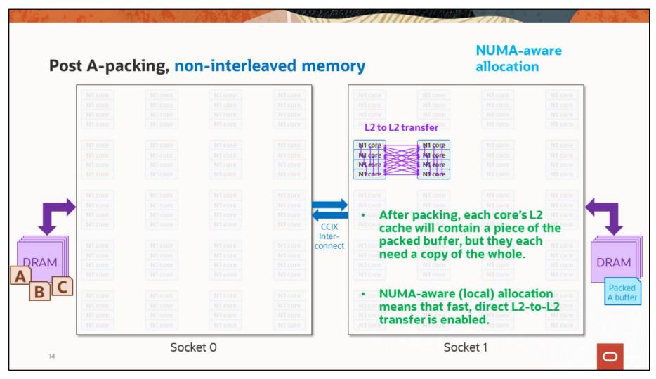
During A packing, a group of threads like that shown collaborate to pack their shared "packed A" buffer. With NUMA-aware allocation, the buffer will be allocated to the address space of the socket 1 DRAM, since these threads all live on socket 1.
