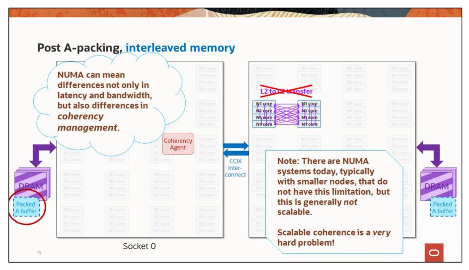
With interleaved memory, the data is striped across both DRAMS. This means that part of the packed buffer is in the socket 0 address space and part is in the socket 1 address space.
