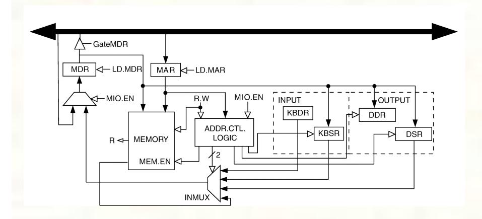
Because of interrupt enable bits, status registers (KBSR/DSR) must be written, as well as read.
