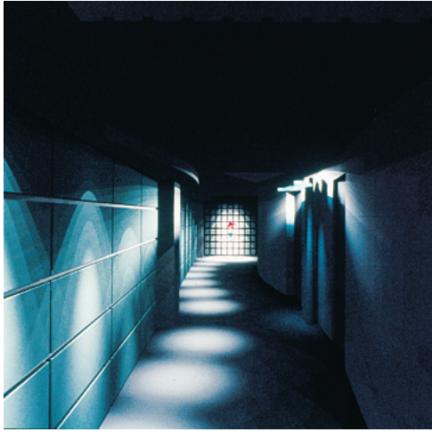
FIGURE 1-17 A hotel corridor that provides a sense of movement by positioning light fixtures along an undulating path and creates a sense of entry by placing a light tower at the entrance to each room. (Courtesy of Skidmore, Owings, & Merrill.)
