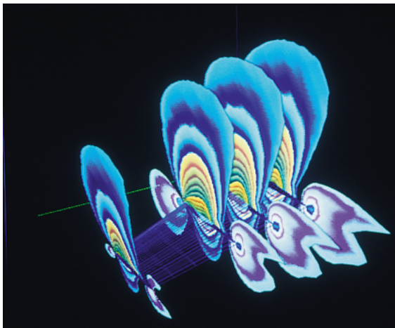
FIGURE 1-33 A fluid-dynamic simulation, showing a color-coded plot of fluid density over a span of grid planes around an aircraft wing, developed by Lee-Hian Quek, John Eickemeyer, and Jeffery Tan. (Courtesy of the Information Technology Institute, Republic of Singapore.)
