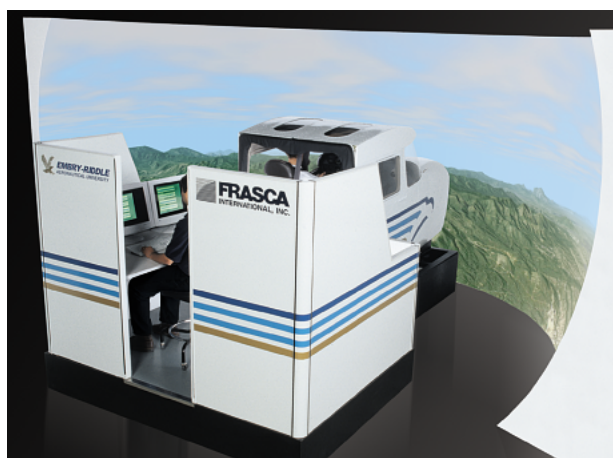
FIGURE 1-47 An instructor's area behind the cabin of a small flight simulator. The equipment allows the instructor to monitor flight conditions and to set airplane and environment parameters. (Courtesy of Frasca International.)
