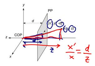
By similar triangles, we can compute how much the *x* and *y* coordinates are scaled:
