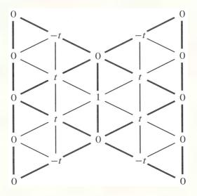
Setting t=0 gives the original polyhedron, and increasing small values of t makes the surface smoother, until t=1/8 when the surface is provably  $G^1$ .
