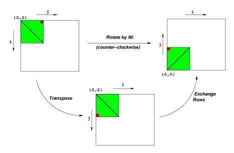
Figure 1: Rotation of an image by  $90^\circ$  counterclockwise
