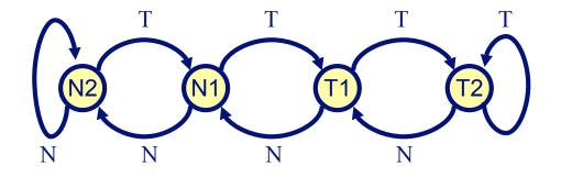
This is a sequential logic circuit that can be formulated as a state machine
