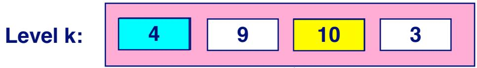
Smaller, faster, more expensive device at level k caches a subset of the blocks from level k+1
