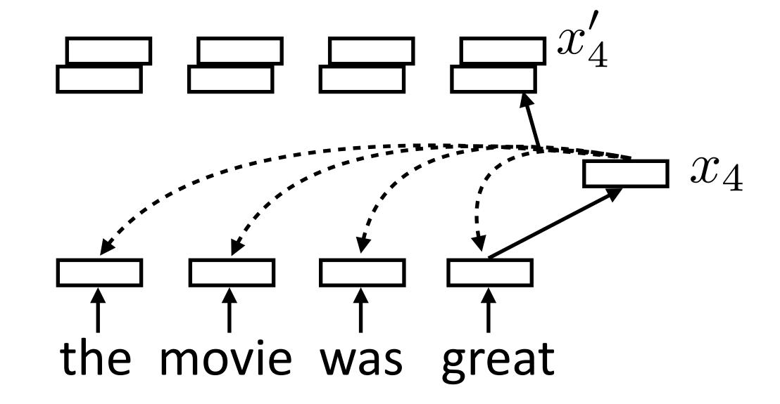
Multiple "heads" analogous to different convolutional filters. Use parameters  $W_k$  and  $V_k$  to get different attention values + transform vectors
