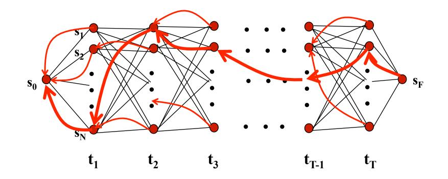
Most likely Sequence: s<sub>0</sub> s<sub>N</sub> s<sub>1</sub> s<sub>2</sub> ... s<sub>2</sub> s<sub>F</sub>
