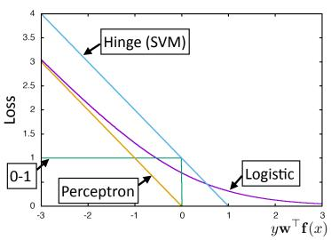
**Figure 2:** Loss functions for perceptron, logistic regression, and SVM (the hinge loss). 0-1 loss, the "ideal" classification loss, is shown for comparison.
