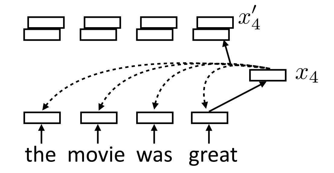
Multi-head self attention: we are going to replicate this machinery several times with different parameters
