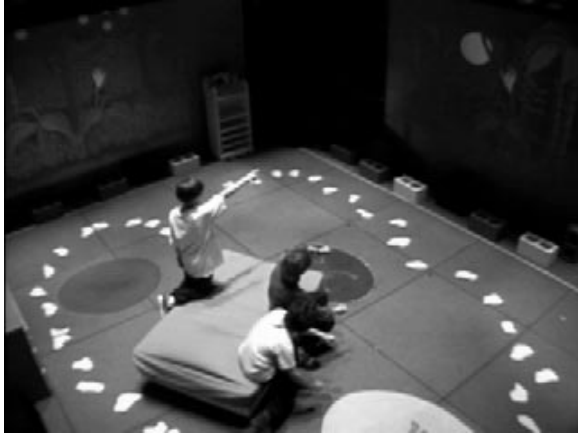
Figure 8: The KidsROOM interactive play-space. Using a modified version of temporal templates the room responds to the actions of the children. All sensing is performed using vision from 3 cameras.
