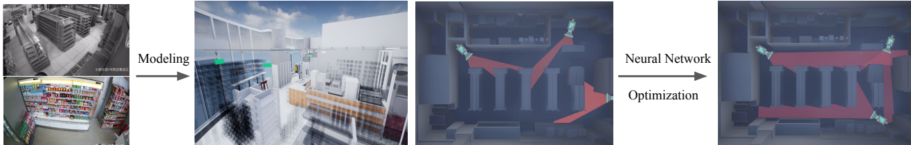
Figure 1: We present a method that optimizes max-coverage camera placement based on learning. Given the real scene model with the areas of interest (marked as black blocks) that require to be covered by a set of cameras, we learn a continuous scoring function and apply continuous optimization on camera poses to improve the global coverage score. In this figure, the red area in the top view of a scene indicates that the coverage increases after optimization.
