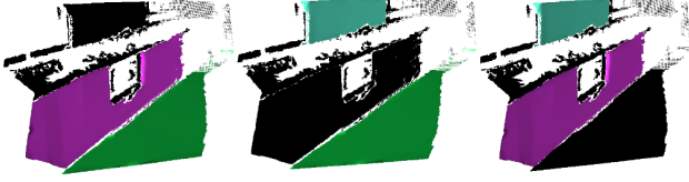
Figure 3. Illustrations of different types of planar relations. (a) Adjacent planes. (b) Perpendicular planes. (c) Parallel planes.
