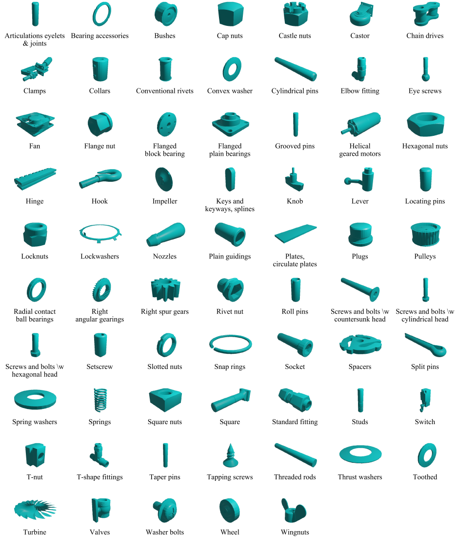
Fig. 10. Samples of Mechanical Components Benchmark (MCB) dataset of a total 68 classes.
