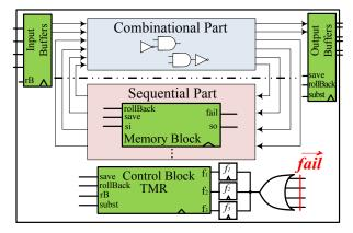
Fig. 4: Transformed circuit for DTR.
