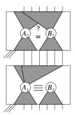
Fig. 1. Speculative reduction simplifies the unrolled netlist.
