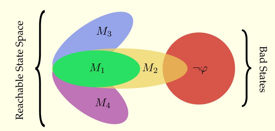
Venn diagram representation of reachable states for a set of models  $M = \{M_1, M_2, M_3, M_4\}$  and bad states  $\neg \varphi$ . Model  $M_2 \not\models \varphi$  since reachable states of  $M_2$  intersect bad states  $\neg \varphi$ . If  $M_1$  is checked before  $M_2$ , the checker run for  $M_2$  can reuse the already explored and verified state space of  $M_1$ .
