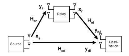
Fig. 1. Wireless relay channel.
