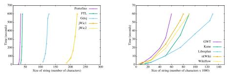
Fig. 8: Running times for exponential vulnerabilities (left) and super-linear vulnerabilities (right) for different input sizes.
