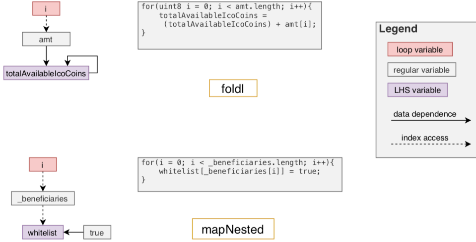
Figure 8: Modeling the semantics of loops using program dependence graph.
