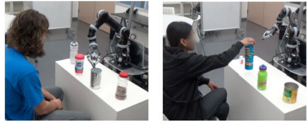
Figure 12. Left: the robot guesses an object described by a human participant as silver, round, and empty. Right: a human participant guesses an object described by the robot as light, tall, and tub.
