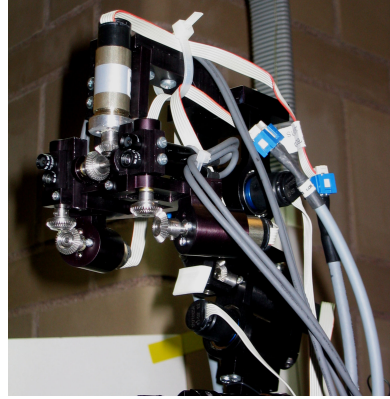
Fig. 2. The robot's head-neck assembly, housing a four camera vision system and providing a total of 7 DOFs.
