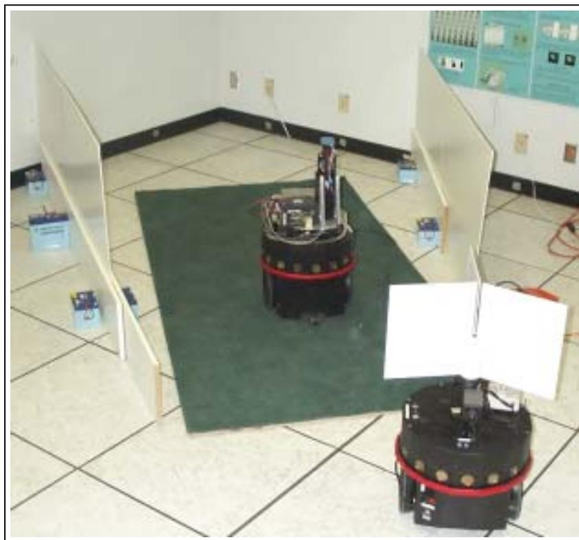
Figure 9: Measuring the odometry error on carpet.
