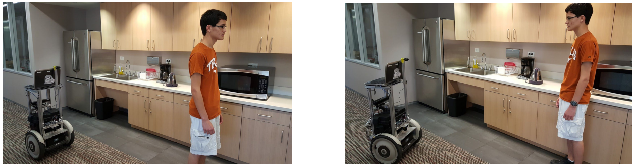
Figure 3: Robot first orienting itself toward its target (left), then moving toward its target (right).
